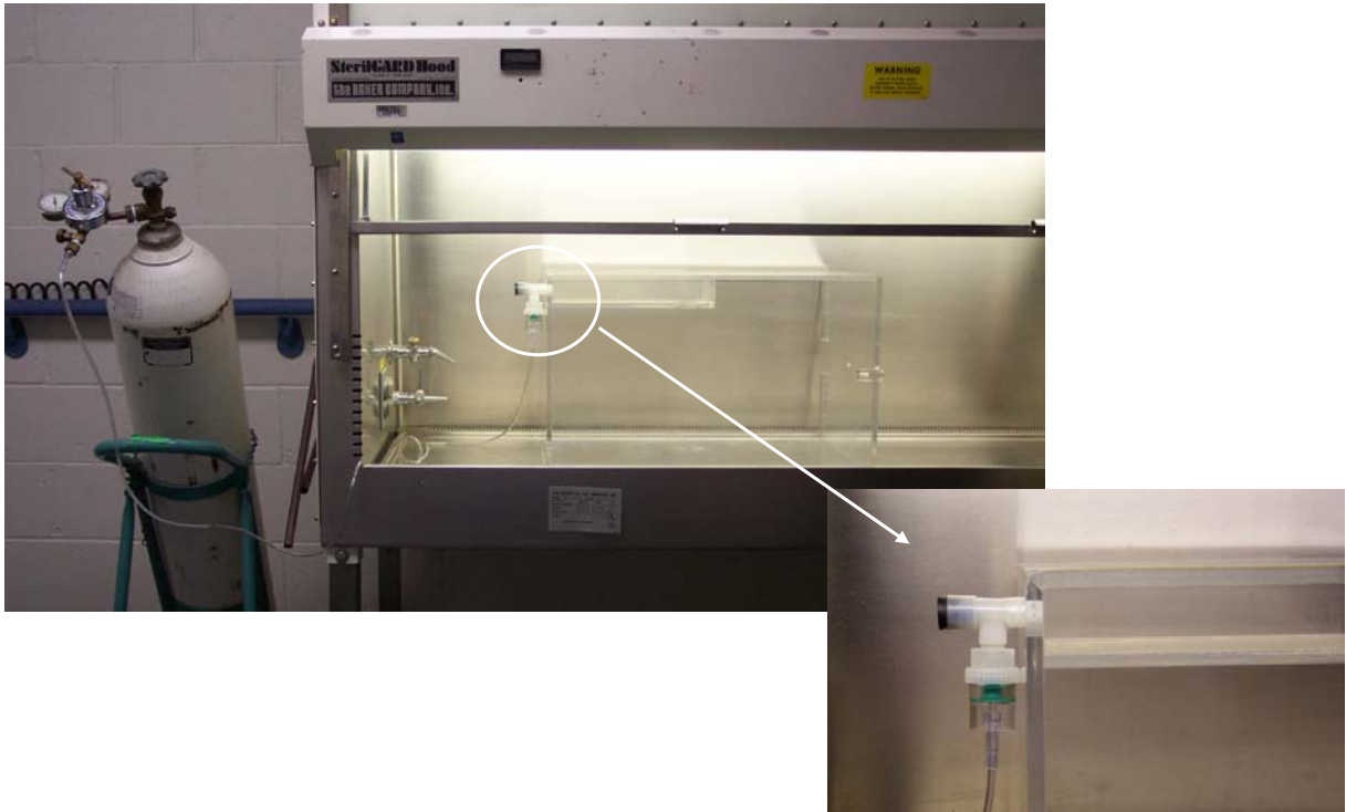
Figure 1. Acrylic Inhalation Chamber Apparatus for Aspergillosis
